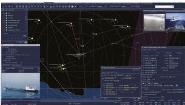
MILSOFT's Mil-CMS combat management system, which features an Open Architecture Computing Environment (OACE), is actively used on the corvettes of the Turkish Coast Guard.
